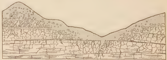
FIG. 21. — Diagram showing the relation of residual soil to underlying rock. (U. S. Geol. Surv.)
